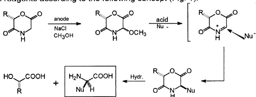
**Figure 1:** Concept for the application of chiral 3-methoxy-2,5-morpholinediones as cationic glycine equivalents.
