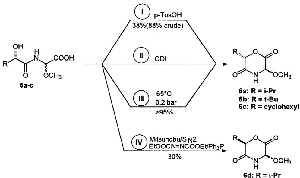
**Figure 5:** Cyclization methods for the open-chain methoxylated dipeptolide **5** (p-TosOH = *p*-toluene sulfonic acid; CDI = carbonyl diimidazole).
