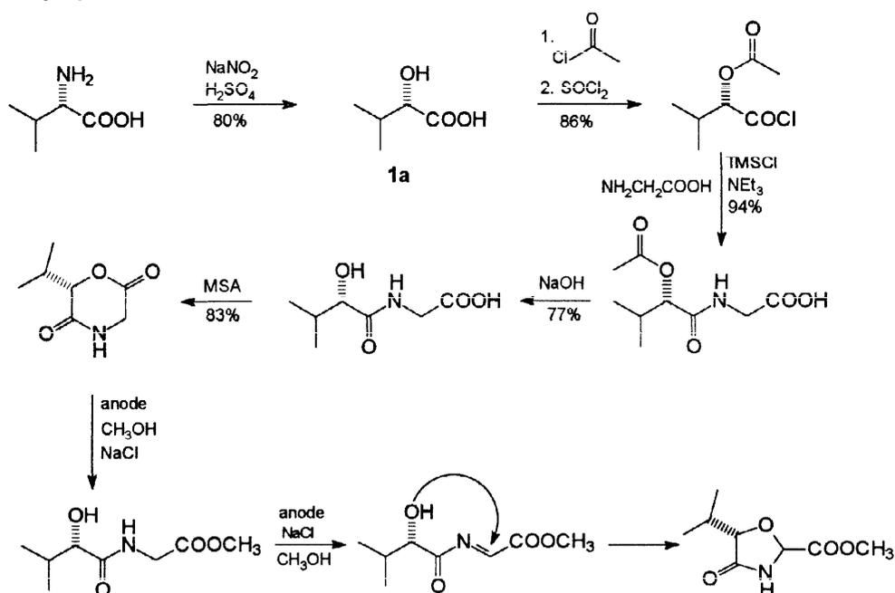
**Figure 2:** Attempted synthesis of a 6-substituted chiral 3-methoxy-2,5-morpholinedione via indirect electrochemical methoxylation of a cyclic dipeptolide.
